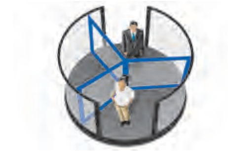
Three/Four-wing revolving doors ← The door wings of the three/four wings revolving doors are fixed to the central axis which can drive the door wings.
