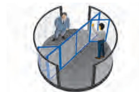
Two-wing automatic revolving doors ← The door wings of two-wing doors are fixed to the H-girder which can drive the door wings.
